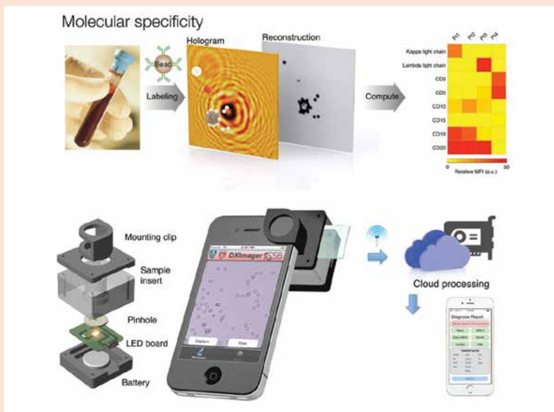
FIG. 2 (PROC NATL ACAD SCI. 2015;112:5613). Design and implementation of the D3 smartphone diagnostic system. (Top) Blood or fine needle aspirate samples are labeled by molecular-specific microbeads and imaged without washing steps by the real-time holographic method. The images of cancer cells are reconstructed from recorded holograms using a multi-core graphics processing unit (GPU) implemented computing systems for rapid calculation. The detection results are quantitative. (Bottom) Schematic of the holographic, D3 detection system mounted on a smartphone. Mathematical reconstruction of holograms is done via cloud processing in seconds and results in diagnostic reports.
