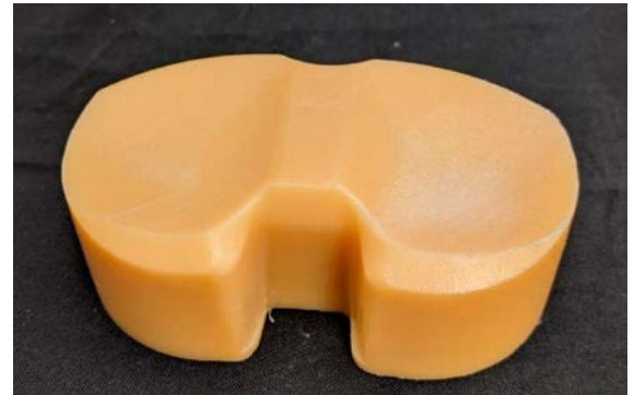
The first prototype of a gentamycin sulfate eluting polyethylene tibial knee spacer intended to treat periprosthetic joint infection in total knee replacement patients.
