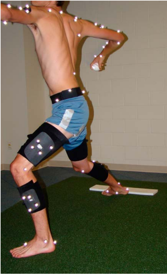
Markers are placed on a high school pitcher to allow optical motion analysis cameras to create 3D visualizations of pitches.
